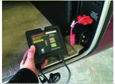
In our view, a battery tender is the best investment you can make to prolong the life of a battery. The \$240 BatteryMinder from VDC Electronics was specifically calibrated for aircraft batteries and there are models appropriate for Gill, Concorde and Hawker-Odyssey batteries.
